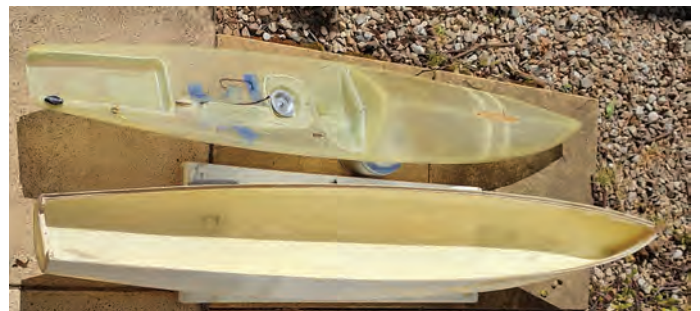
The hull and deck are almost ready for joining after a bit more work on a keel box.
